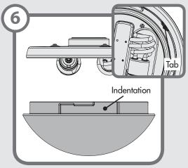
Installing the globe (sold separately)- Position the indentations in the outer rim of the globe so that they line up with the tabs on the inside surface of the light fixture rim. Carefully lift the globe up inside the light fixture as far as it will go. Rotate the globe in a clockwise direction until it is held tightly in place by the four tabs.
